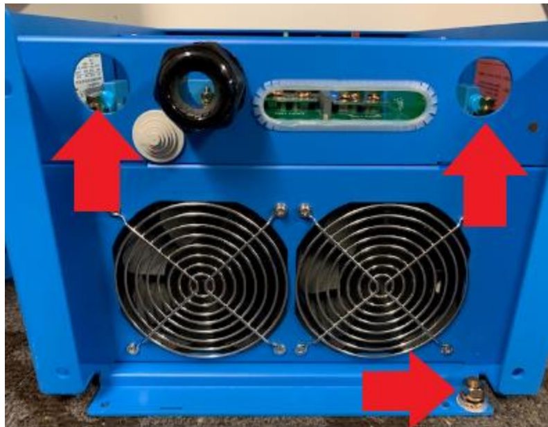
Figure 23-5kVA Ground Connection Points
