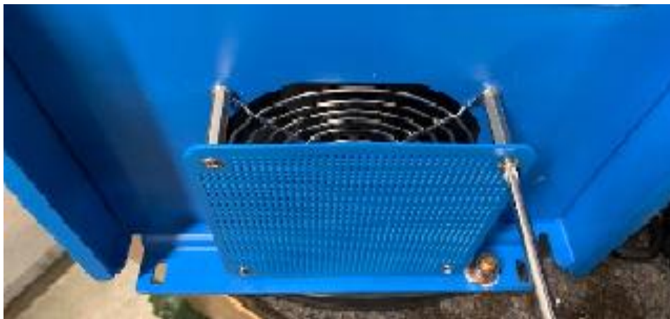
Figure 4-3kVA Blue Fan Cover Plate Installed
