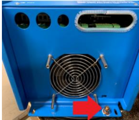
Figure 22-3kVA Ground Connection Point
