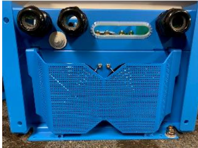
Figure 6-5kVA Blue Fan Cover Plate Installed
