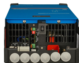
MultiPlus 2000 VA (bottom cover removed)
