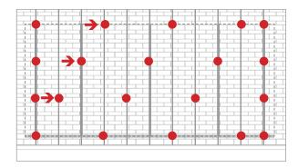
**TO STAGGER ATTACHMENTS:** Shift each subsequent row of attachments one rafter over.
