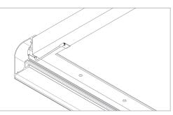
**Trimrail Bonding Alternate Method:** Attach a bonding clip from the Trimrail<sup>™</sup> to an adjacent module. Fully seat bonding clip until radius portion is in contact with Trimrail<sup>™</sup> mating surface and module flange.
