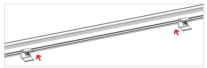
**INSTALL MODULE CLIPS ON TRIMRAIL:** Attach module clips to Trimrail using 3/8" T-bolts and Tri-drive or serrated flange nuts. A minimum of two clips are required per module. Refer to SFM D&E guide and U-builder for required position and quantity of module clips. NOTE: module clips may be pre-installed on trimrail prior to attaching trimrail to roof attachments
