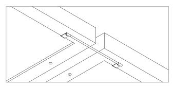
N/S Bonding Alternate Method: Fully seat bonding clip on each module flange to provide bond across N/S module gap.
