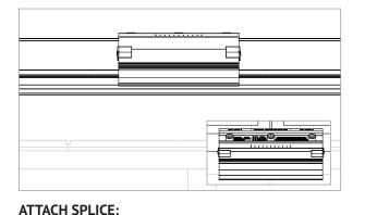
Attach splice at intersection of two (2) modules.
