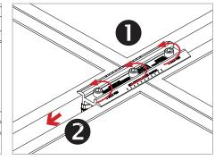
**SLIDE FLOATING SPLICE:** 1. Loosen (3) cap bolts approx. 3 turns. 2. Slide entire floating splice away from module being removed.
