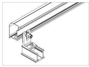
ATTACH TRIMRAIL TO ROOF ATTACHMENT: Attach rail using 3/8" hex bolt & Tri-drive or serrated flange nuts. Make sure Trimrail<sup>TM</sup> is level across all Trimrail<sup>TM</sup> roof attachments. After rail is level, tighten channel clamp bolts to secure Trimrail<sup>TM</sup> roof attachments to channels.
