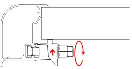
SECURING TRIMRAIL<sup>™</sup> WITH FLOATING TRIM CLAMPS: Installation of floating trim sections may occur before module is secured. Floating Trim Clamp captures module flange when nut is tightened to 20 ft-lbs as shown above.
