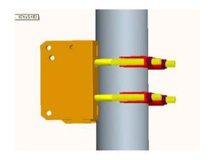
Step 3 - attaching the panel/arm assembly to the bracket
