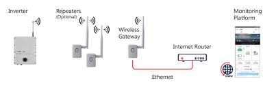
Scenario B: Multiple inverters, wired connection<sup>(3)</sup>
