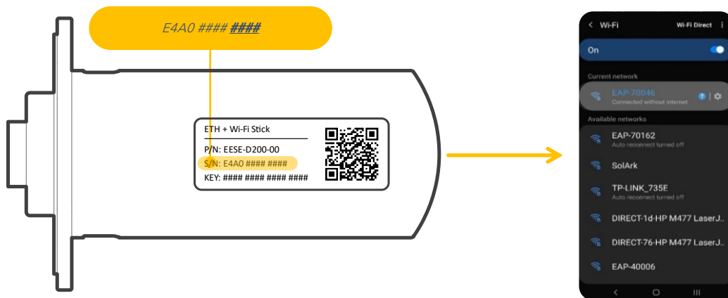
Figure 38: E4A0-##### serial number and EAP network
