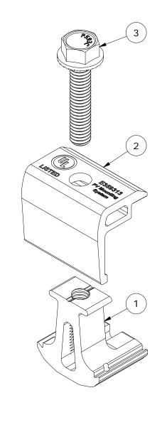
CLAMPS FIT 30-46MM THICK MODULE FRAMES
