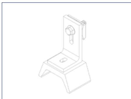
Corrugated Roof Block Attachment Roof attachment for sinusoidal corrugated metal roofs including roof block, L foot, and hardware
