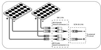
Fig. 5. Connecting two adjacent solar panels in parallel
