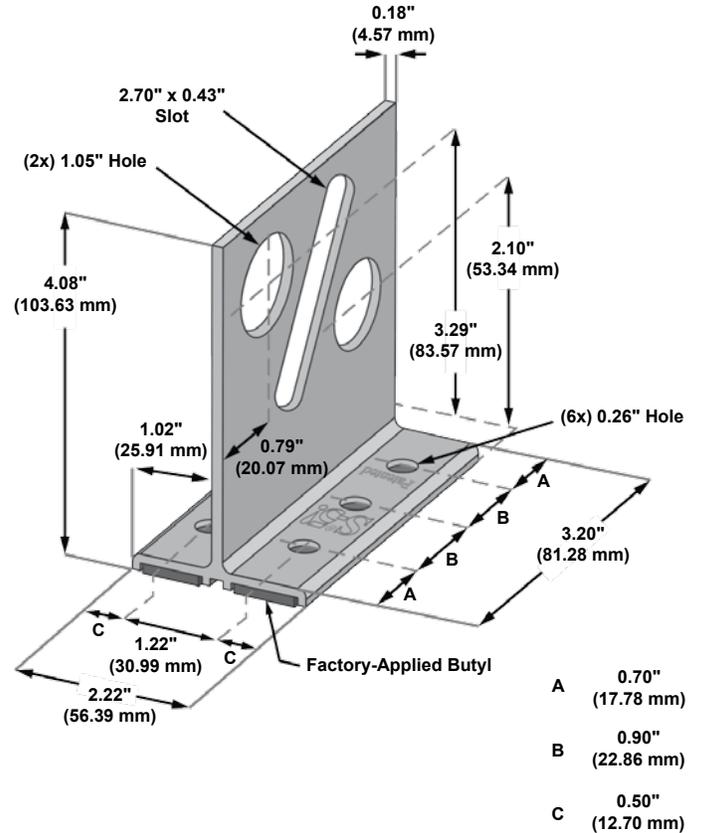
6 holes are provided for versatility. Some installations require only 2 fasteners. See the load table on the S-5! website and the installation instructions for more details.
