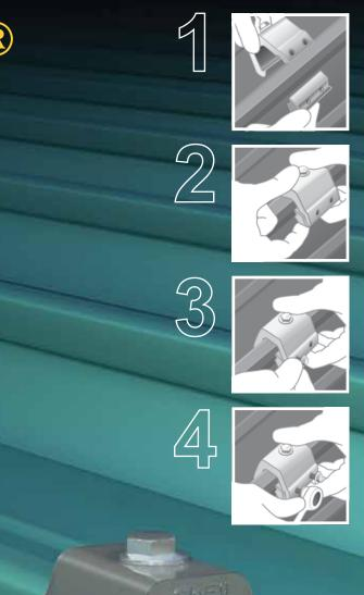
The S-5-K Grip<sup>™</sup> was specifically developed to fit Klip-Rib<sup>®</sup> and other bulb snap-together seams.
