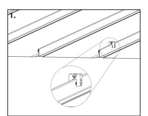
**2. Slide S-5-Tab CF into channel of GRIPPERFIX Strut:** Slide an equal number (to clamps) of tabs into the channel as shown in **(Fig 2a)**. Be sure that the surface with slotted hole is oriented upward. **(Fig 2b)**.
