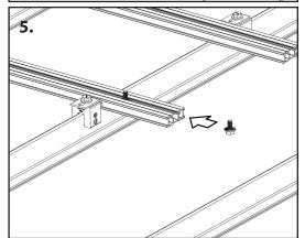
**6. Place ancillary object to be mounted over M8 Bolts and complete assembly:** Place the mounting holes on the base of the object being mounted over the inserted M8 bolts. Tighten the provided nuts onto the bolts. Check and tighten any remaining hardware. **(Fig. 6)**
