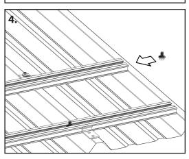
**4. Slide M8 x 16 or 20 mm Bolts into Bolt Slot:** Slide the appropriate number of M8 bolts into the top slot of each GRIPPERFIX Strut (**Fig. 4**). Position these bolts such that they align with mounting holes of the object to be mounted.
