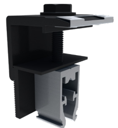
Image 2.4.10-1 Universal end clamp w/WEEB-BMC [96 in-lbs (11 N-m)]
