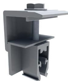
Image 2.4.9 Universal end clamp [96 in-lbs (11 N-m)]
