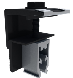
Image 2.4.10-1 Universal end clamp w/WEEB-BMC [96 in-lbs (11 N-m)]
