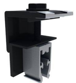
Image 2.4.10-1 Universal end clamp w/WEEB-BMC [96 in-lbs (11 N-m)]
