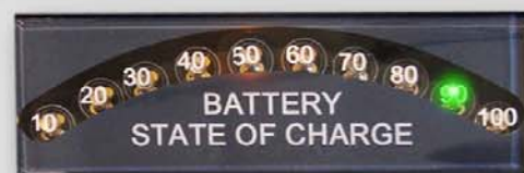
Batteries have a 90% charge
