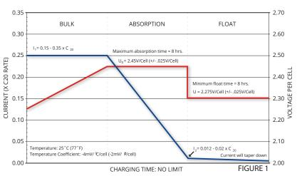
The initial charge current is recommended to be set at  $0.20 \times C$  in order to fully charge the batteries within a reasonable amount of time. It can be set lower; however, please be aware that charge time will increase so make sure the batteries have enough time to fully charge before being put back into service. Fullriver batteries have a low internal resistance allowing them to be charged at a higher current, therefore faster, than conventional flooded/wet batteries.
