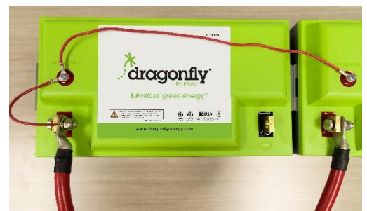
Figure 7: Top view of daisy chained heat-enable post
