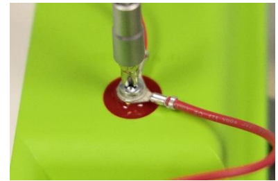
Figure 13: #8 ring terminal onto the heater enable post
