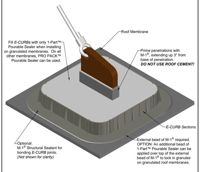
A minimum 1" space is required between all penetrations and the interior wall of all E-CURBs.
