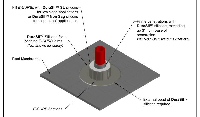
A minimum 1" space is required between all penetrations and the interior wall of all E-CURBs.
