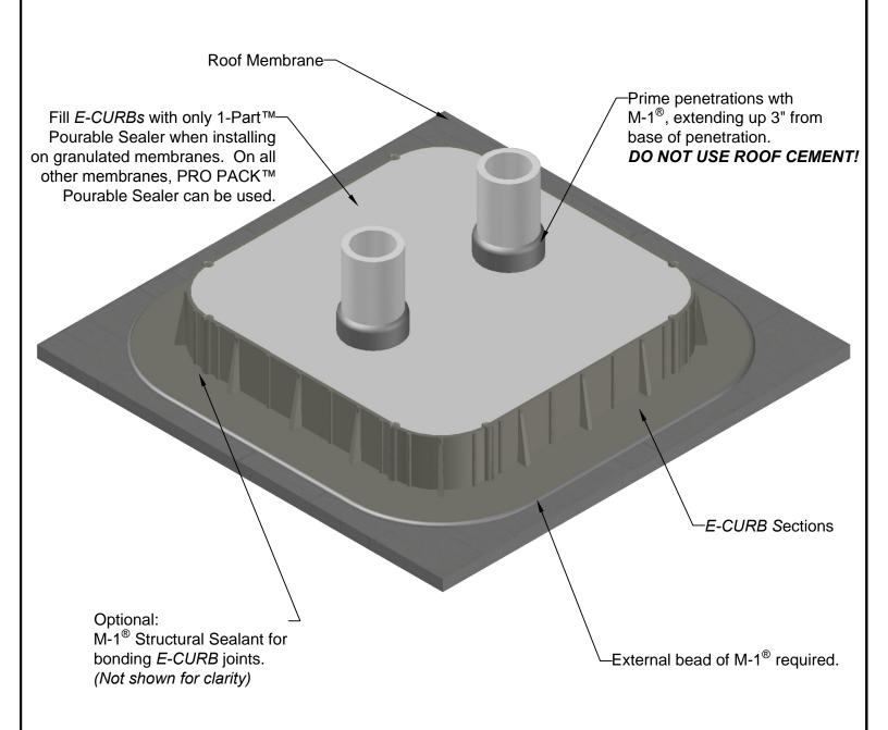
A minimum 1" space is required between all penetrations and the interior wall of all E-CURBs.
