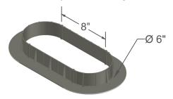
To figure volume of a round curb: multiply (radius squared x 3.14 x depth) x (quantity of curbs needed) then divide by 231 (in<sup>3</sup>/gal) to get the number of gallons needed to fill the curb.
