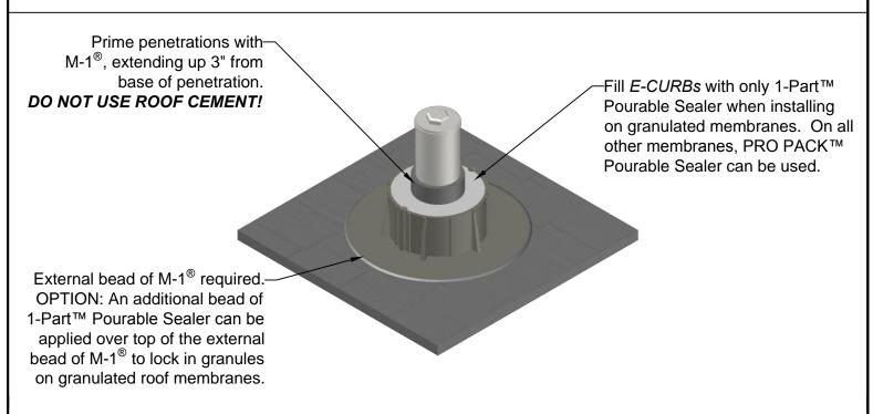
A minimum 1" space is required between all penetrations and the interior wall of all E-CURBs.
