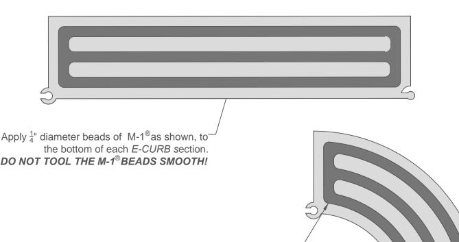
Apply <sup>1</sup>/<sub>4</sub>" diameter beads of M-1<sup>®</sup> as shown, to the bottom of each *E-CURB* section.
