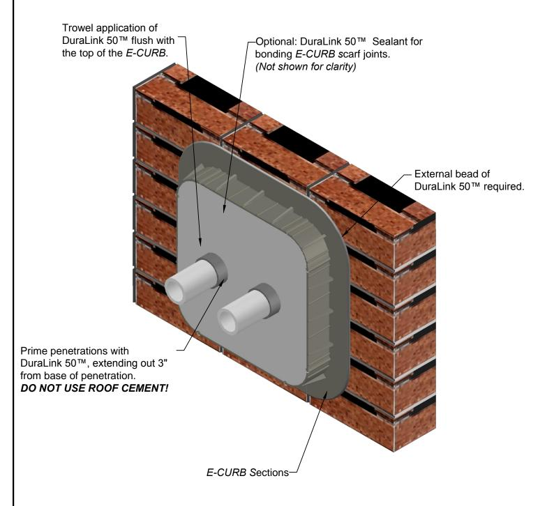
A minimum 1" space is required between all penetrations and the interior wall of all E-CURBs.
