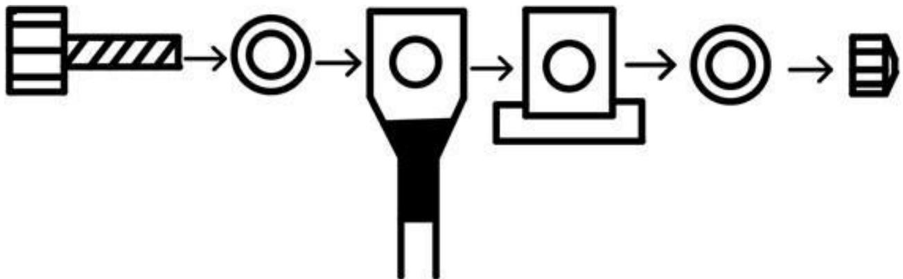
*Figure 1: Proper order of hardware to connect cables. When going from left to right in the diagram the correct order is: bolt, washer, lug, terminal, washer, and nut. If multiple lugs are used, they should be on the same side of the terminal.*
