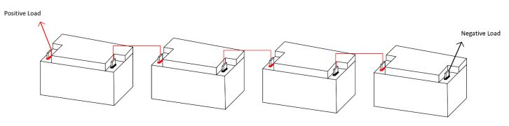
Figure 4.2: Four 1250 Batteries Connected in Series to create a 48V 50Ah Battery Bank \*Individually charge each battery to 100% prior to connecting your battery bank in series\*
