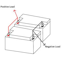
Figure 3.1: Two 1250 Batteries connected in Parallel to create a 12V 100Ah Battery Bank
