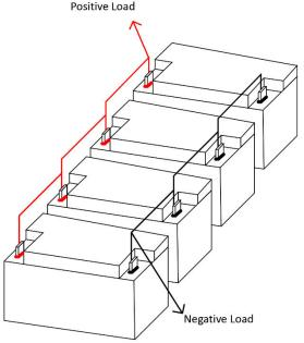
Figure 3.2: Four 1250 Batteries connected in Parallel to create a 12V 200Ah Battery Bank
