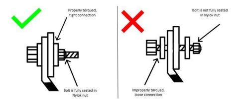
Figure 2: Proper and Improper Terminal Connections
