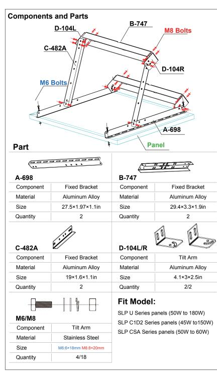
\*(M6) all 4 mounting bolts will be used to install A-698(fixed bracket) to the PV module frame. Place 1 mounting bolt on each of the 4 sides of the PV module frame.
