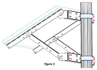
**Step 2.** Gather fixed bracket (C-482A) and align with designated holes along the frame of the PV module for the desired tilt angle. Install one mounting bolt on each side to connect to the PV module frame. Then install the fixed bracket (B-747) along with tilt arm (D-104L/R) to fixed bracket (C-482A). Once done, the bottom portion of mounting kit will be completed.
