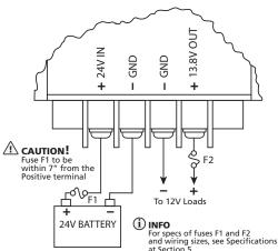
Fig 4.1 Installation Diagram
