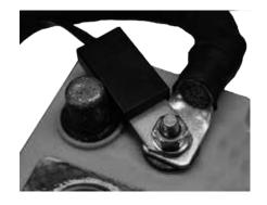
Fig 2.5(a) Temperature Sensor Model EVO-BCTS
