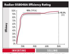
Typical Efficiency Rating: Real world efficiency with variable loads • GS8048A: 93% CEC Efficiency Rating: Most stringent US rating • GS8048A: 92.5%
