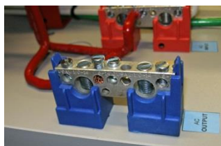
Replace the Busbar and press into place
