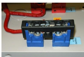
Replace wiring cover. Black cover shown here
