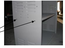
**Step 2**: Install eight #10 x 3/8" Flat head Philips SS sheet metal screws front and back to attach sides to shelves. Additional shelves may be purchased to accommodate other configurations.
