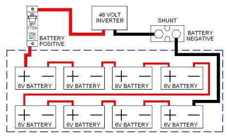
This configuration uses 6 volt sealed batteries that result in only one string. This is a 48 volt battery bank. You could add 3 more cabinets and have only 4 paralleled strings.
