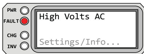
Figure 5-22, High Volts AC Fault
