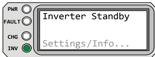
Figure 5-5, Inverter Standby Mode
