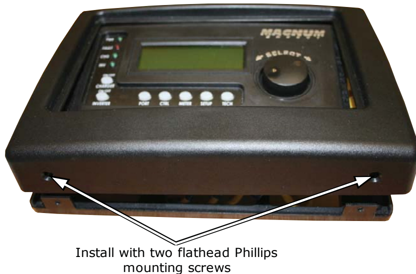
Figure 2-11, Installing the Router Cover
