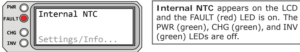
Figure 5-35, Internal NTC Fault
