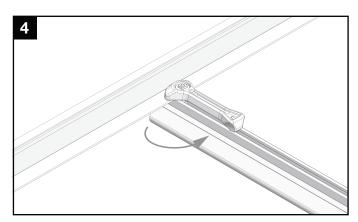
Rotate handle with an upwards motion until CAMO snaps into rail channel. Ensure Camo bonding pins are fully seated on top of module frame.
