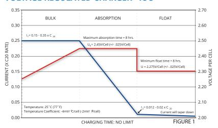
The initial charge current is recommended to be set at  $0.20 \times C$  in order to fully charge the batteries within a reasonable amount of time. It can be set lower; however, please be aware that charge time will increase so make sure the batteries have enough time to fully charge before being put back into service. Fullriver batteries have a low internal resistance allowing them to be charged at a higher current, therefore faster, than conventional flooded/wet batteries.
