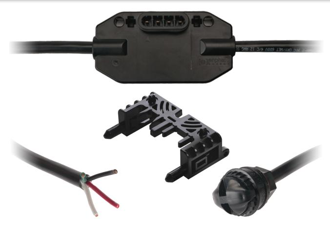
The Engage Cable is a continuous length of 12AWG cable with pre-installed connectors for Enphase Microinverters to plug into. The cable is handled like standard outdoor-rated electrical wire, allowing it to be cut, spliced and extended as needed.
