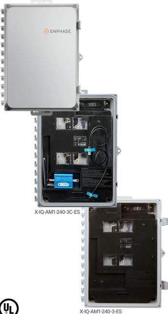
The **Enphase IQ Combiner 3-ES/3C-ES**™ with Enphase IQ Envoy™ and integrated LTE-M1 cell modem (included only with IQ Combiner 3C-ES) consolidates interconnection equipment into a single enclosure and streamlines PV and storage installations by providing a consistent, pre-wired solution for residential applications. It offers up to four 2-pole input circuits and Eaton BR series busbar assembly.
