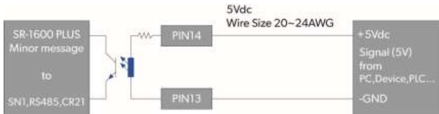
Figure 9-4. Application diagram of dry contact pin14~13(Minor)
