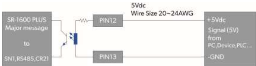
Figure 9-3. Application diagram of dry contact pin12~13(Major)
