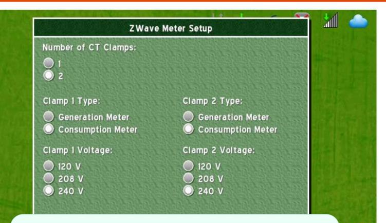
Select the mode for each clamp and the voltage of the circuit it is clamping. Note that the voltages are scaling factors, the voltage the meter is plugged into with the supply lines must not exceed 150 Vrms)
