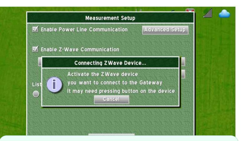
Press the button the zWave device to pair it, device must be within range of Gateway. Repeaters can be used to extend the range, but repeaters must be paired in proximity to the Gateway, we first pair a repeater
