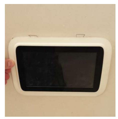
Warning! Make sure removable rear socket is connected to ROMEX and plugged into unit, and rear cover is fixed back in place, before installing in wall
