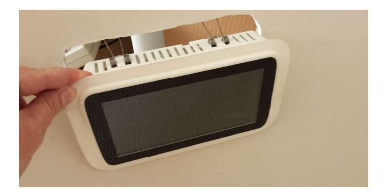
Warning! Make sure removable rear socket is connected to ROMEX and plugged into unit, and rear cover is fixed back in place, before installing in wall
