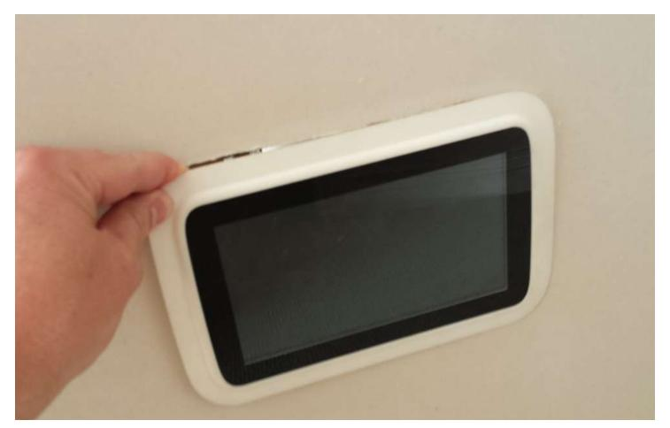
Warning! Make sure removable rear socket is connected to ROMEX and plugged into unit, and rear cover is fixed back in place, before installing in wall
