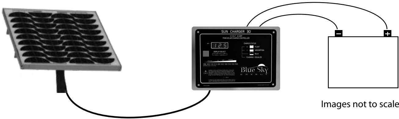
Typical illustration of solar panel to Sun Charger 30 to Battery
