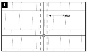
Locate rafters and snap vertical and horizontal lines to mark flashing locations. Drill 1/4" pilot holes, then fill with roofing manufacturer's approved sealant.
