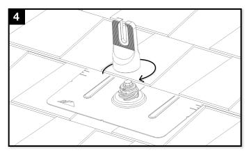
Place Cap onto flashing in desired orientation for E/W or N/S rails and rotate 180 degrees. FlashFoot 2 is now installed and ready for IronRidge XR Rails.
